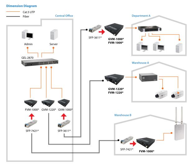
\* In above example diagram, converter modules at local and remote ends should be paired for proper connectivity, and the distance mainly depends on cable and transceiver selection accordingly.
